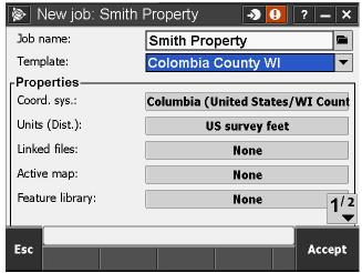
Step 13. Templates are saved in the "**Trimble Data/System Files**" folder. Templates can be copied from one collector to another if the versions of Trimble Access are the same. My Trimble Access can be used to convert a template to the latest version.
