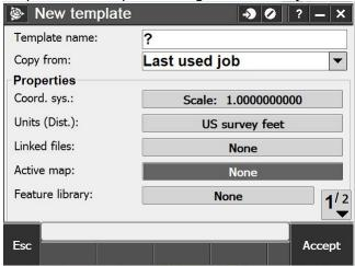
Step 6. Name the template, you can "**Copy from**" an existing template if you have one that is similar to the one you wish to create. For example, if an existing template is set to the correct coordinate system and just the geoid model needs to be changed.
