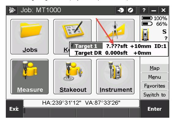
Step 3. Under the drop down menu for prism type select VX/S Series MultiTrack
