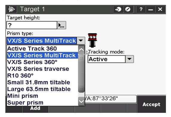
Step 4. Click on the drop down menu for **tracking mode**. This is where you will select the mode based on what you are trying to do. Most applications will be Active track. When you need more accurate vertical results, it is best to select Semi-Active. Passive is rarely used but is always an option if you run out of battery power or when interference is highly unlikely.
