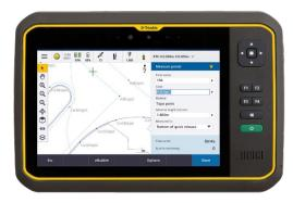
real time using Microsoft® Office software applications or third-party developed software. The T7 tablet has a flexible modular system for expansion and an internal professional GNSS receiver for accurate real-time positioning. Featuring a 7-inch sunlight readable screen, hot-swappable batteries, and military certified rugged exterior, the T7 tablet is designed to work in the toughest environments for maximum efficiency and productivity.
